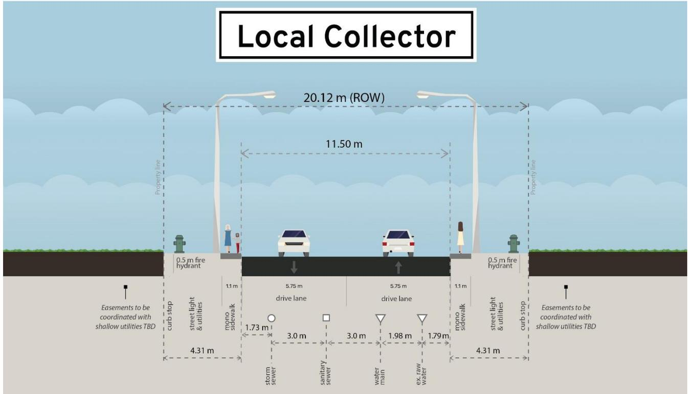
Figure 9 | Residential Boulevard Road Cross-Section with Utilities
